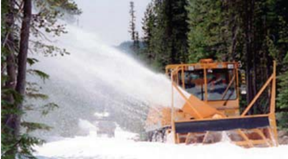
Consider the size of snowplows when determining road width on roads receiving lots of snowfall.
