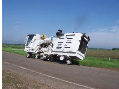
Milling machine tipping on low side of elevated horizontal curve
